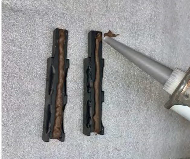
1. Apply cement to the back of the two spacers.
