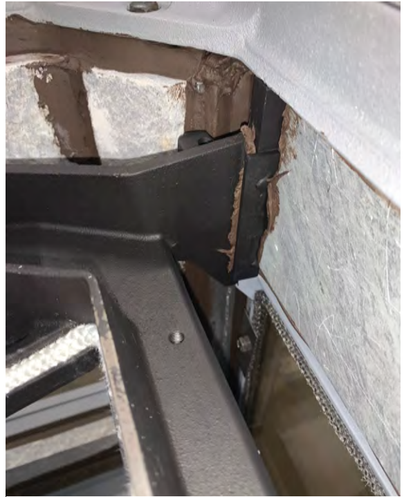
The front rails of the combustor pan fits into the cemented channel in the spacer.
